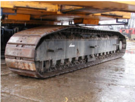
Side track components are Cat. For the 80, the undercarriage is Cat B7 design and for the 2020, B8. This means that you are getting the heaviest components for the class of machine.
