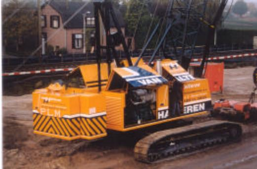
Drop ball is one of the simplest yet most destructive operations you can put a crane into. Every cycle is a shock load. Making matters worse, people generally use machines which are undersized for the work and in reality are two rope, friction machines built for lift crane service.
