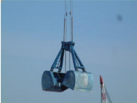
The right and left lay ropes offer the advantage that the clam is very stable and does not require a tagline. This is very important if you are unloading ships where the tagline rubs on hatch coamings and in dredging operations where the clam extends well below the base of the crane. In standard configuration, a 4-rope crane can dig as much as 100ft below the base of the crane.
